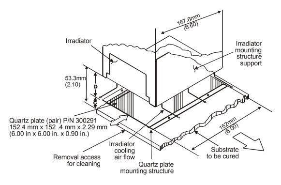
Figure 8. Quartz Plates - Example Mounting Design
